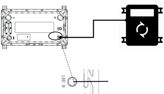
B: When multiple batteries are used in series or parallel, the external device communication line needs to be connected to the battery Link in;
