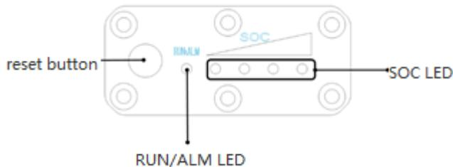
The battery display panel has 1 fault/running light, 4 SOC indicator lights, and 1 button: the usage method is as follows
