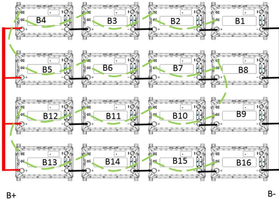
For example: 16 12.8V120Ah batteries, 4 in series & 4 in parallel ---- System voltage:  $12.8V * 4=51.2V$
