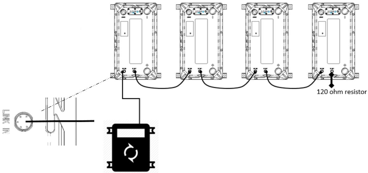
User can use an external communicated cable (optional) to connect to batteries and other device via CAN bus. This allows for communication between the battery and the load or charger, making it more efficient to use the battery. This is also beneficial for understanding battery faults. If you have more questions about the CAN bus, please contact Epoch for technical support.
