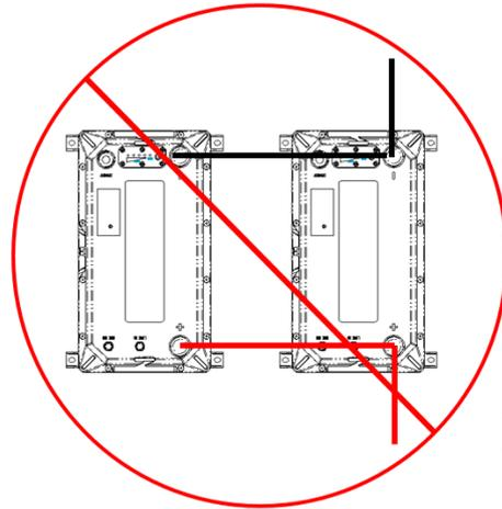
**!** Do not output positive and negative poles on the same battery, which may damage the battery.
