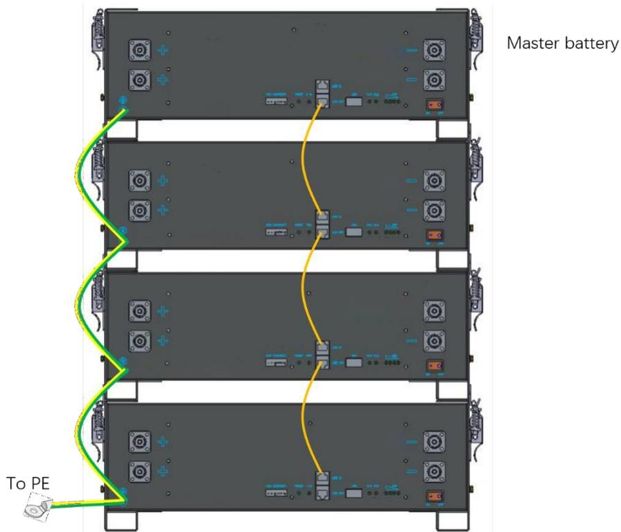
**Note:** the module with empty Link IN port is Master battery
