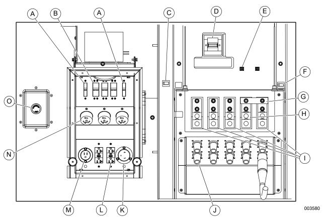
Figure 2-5. Connection Panel Components
