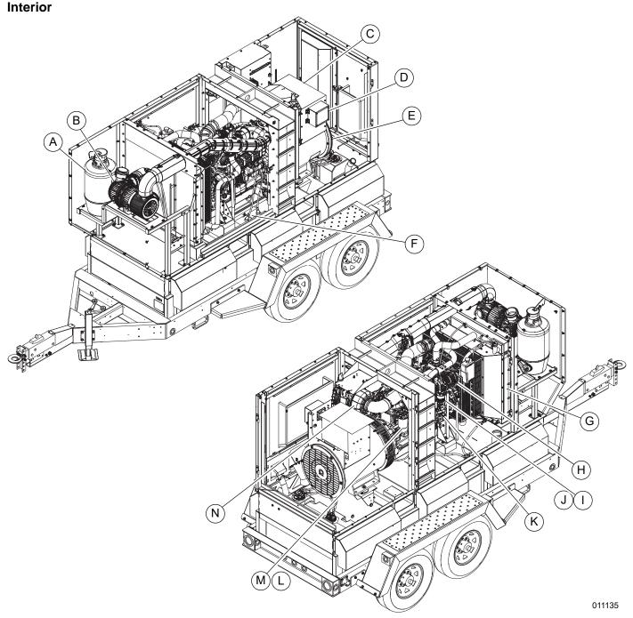
Figure 2-4. Interior Components
