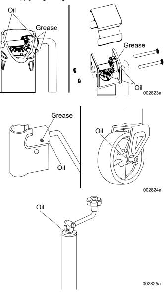
Figure 4-1. Lubrication Points
