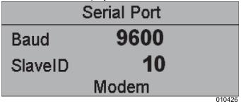
Figure 2-14. Serial Port Page. If modem is not connected, RS232 displays in place of Modem.
