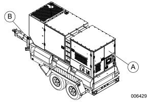
Figure 2-2. Unit ID and VIN Tag Locations
