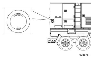
Figure 3-12. Emergency Stop Switch
