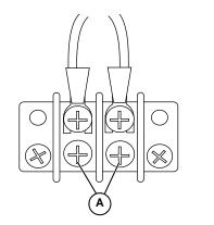
Figure 3-2. Remote Start Terminal Block
