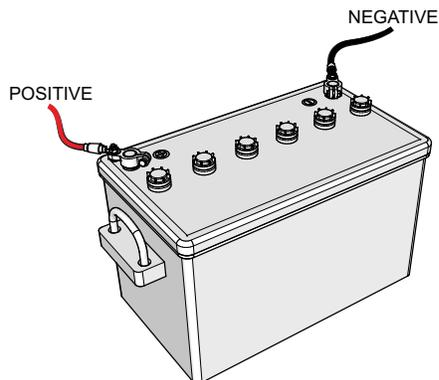
Figure 38. Battery Connections
