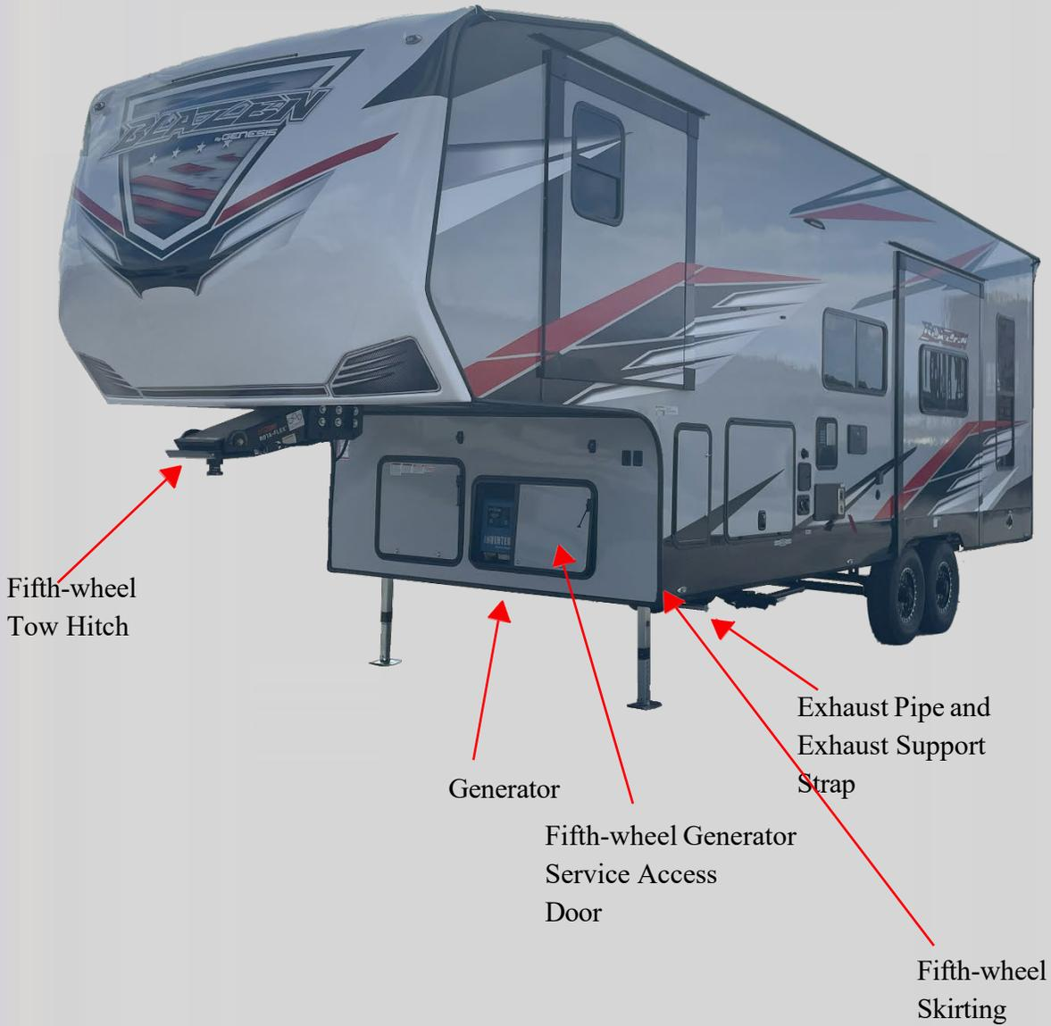
Exhaust should be installed so the horizontal portion of the Exhaust Pipe is level. When possible, downpipe should be omitted to maintain a clearance minimum of 76.2 mm or (3") and maximum of 101.6 mm or (4") from bottom of fifth-wheel skirting to top of Exhaust Pipe. See [Exhibit 7](#).
