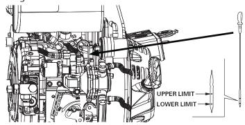
Oil is added to the engine by removing the oil cap and adding oil at this point. After filling the crankcase to the proper level, be sure you properly tighten the oil fill cap. NOTE: This engine generator must be on a level surface before you check or add oil to the system.
