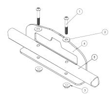
In the bag of parts for the lifting eye, ensure all of the required materials are included: 2 qty - 5/16-18 x 2.25 button head socket screws (#1); 2 qty - washers (#2); 2 qty - .3125-18 flange (#3); 1 qty - lifting eye (#4).
