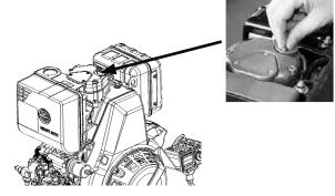
E. Fill to correct level with oil. Reinstall cap. F. Remove the oil filter and dispose of it properly.
