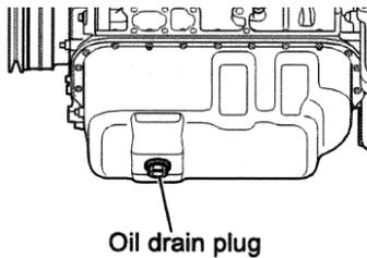
2. Remove the dip stick and remove the engine lubricant oil filter plug.
