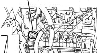
6. Use the dip stick to ensure the level of oil does not exceed the "MAX" limit.
