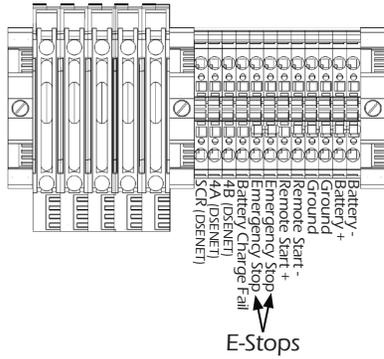
To wire additional emergency stop switches first remove the orange jumper between the two Emergency Stop terminal blocks. Failure to remove the jumper will prevent the remote switches from working properly. Add wires between the terminal block to the new switch(s). The switches must be wired in series for proper function. Test each e-stop after wiring to ensure they function properly.
