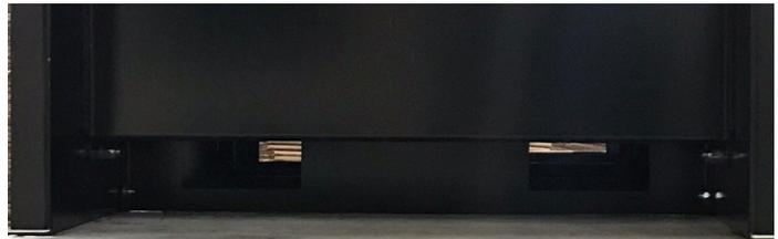
Always use forklifts of a proper rating and with long enough forks to move the generator. As the distance from the forklift mast increases the lifting capacity for the forklift decreases. When lifting from the side the forks should extend the entire width of the unit through the opposite side frame rail.
