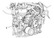
4. After draining the engine coolant, flush the radiator and engine block to remove any rust, scale and contaminants. Then reinstall and tighten the drain plug
