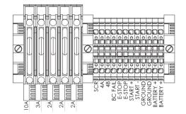
The E-Stop and Remote Start wires have been wired from the controller terminals to the panel for easy installation.
