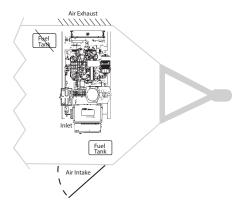
The fuel filler neck is shipped loose and designed to be mounted to an outside wall of the enclosure. The cap will vent fuel vapor if tank pressure to too high.
