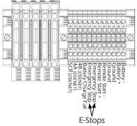
To wire additional emergency stop switches first remove the orange jumper between the two Emergency Stop terminal blocks. Failure to remove the jumper will prevent the remote switches from working properly. Add wires between the terminal block to the new switch(s). The switches must be wired in series for proper function. Test each e-stop after wiring to ensure they function properly.
