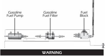
Do not use low-pressure rubber hose for any part of the gasoline system.
