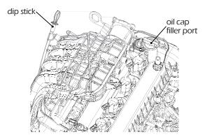
WINCO pipes the oil change to the outside for convenient maintenance.
