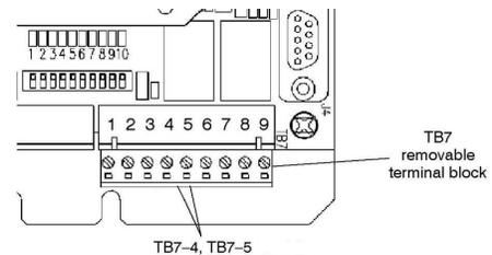
Your DC connection points in the ASCO 185 ATS are terminals "4" and "5" on the interface terminal block. As this is a "DRY" unpowered contract set it set, it makes difference which lead (battery negative #1 or start #23) connect to which terminal.
