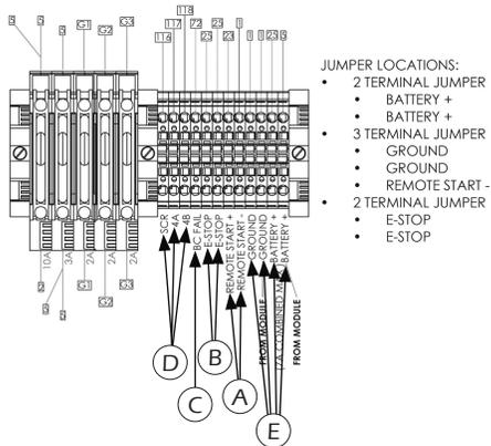
A - Customer Remote Start CONNECTIONS TERMINALS. The two remote start leads from the Automatic Transfer Switch are connected to the two terminals marked 1 & 23. The wire in terminal labeled #1 is Battery Negative/Ground and the wire in the terminal labeled #23 is your Remote Start lead. Closing these two leads together will signal the DSE 7310 MKII to go into an autostart mode and start up the engine generator.
