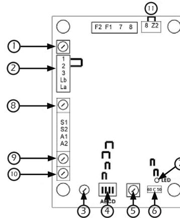
1. VOLTS - Adjust generator output voltage. Clockwise to increase voltage.
