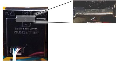
Once open, the battery will be located at the top. Using a needle nose plier, carefully pull out the battery.
