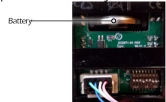
Replace the battery having the POSITIVE (+) side down. Ensure the battery is secured between the battery connections.
