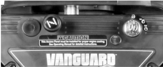
4. Turn the key to the start position. The starter life is improved by using shorter start cycles. Do not operate the starter more than 15 seconds during each minute. Repeat as necessary.
