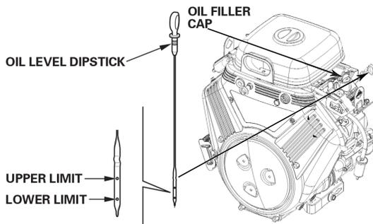
adding oil at this point. After filling the crankcase to the proper level, be sure you properly tighten the oil fill cap.
