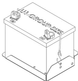
If you intend to use the unit's electric start system, you will need to purchase and install a battery to operate it. A 12 Volt battery, BCI group 26 rated at 500 CCA or larger is recommended for this electric start engine-generator set. Follow the battery manufacturers recommendations for servicing and charging prior to use. Connect the battery to the electric start system using the cables provided.
