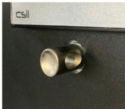
The three positions are 120/240V 1PH, 120/208V 3PH, 277/480 3PH. For 120/240V 3ph, place the selector switch to the 120/208 3PH position and adjust the rheostat to 240V. By doing this you will get 240V, but your single phase voltage will be approximately 139V.
