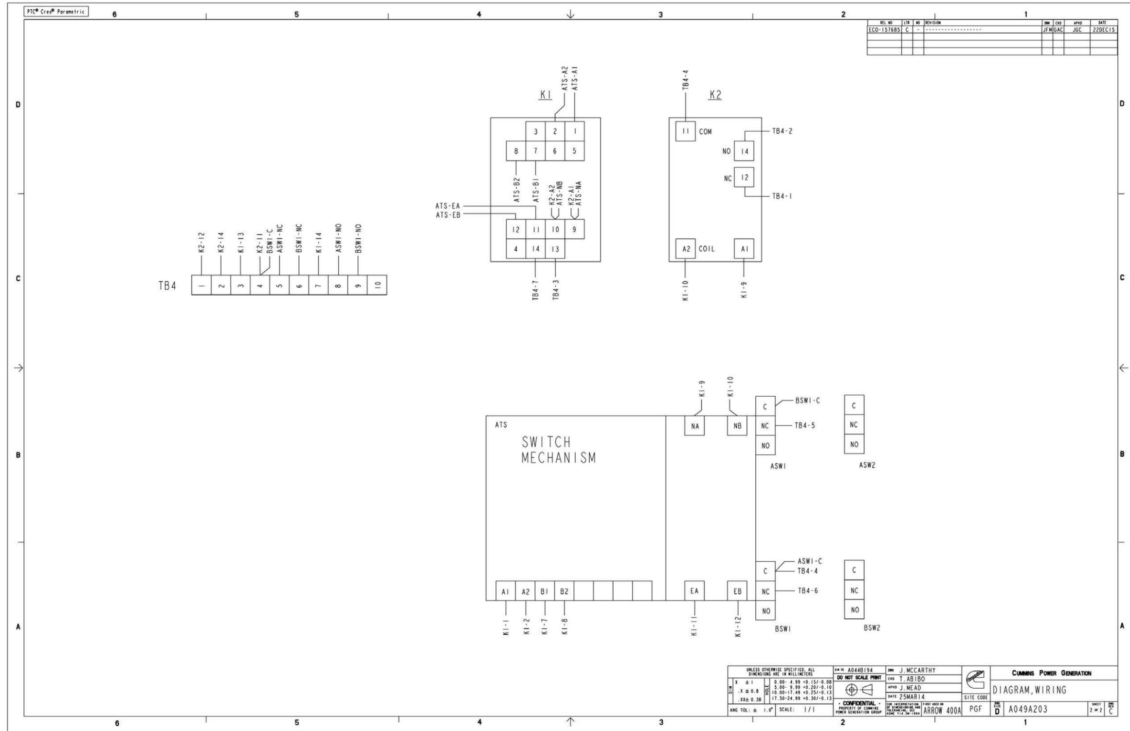
FIGURE 43. RA412N3 AND RA412S3 TRANSFER SWITCH WIRING DIAGRAM (SHEET 2 OF 2)
