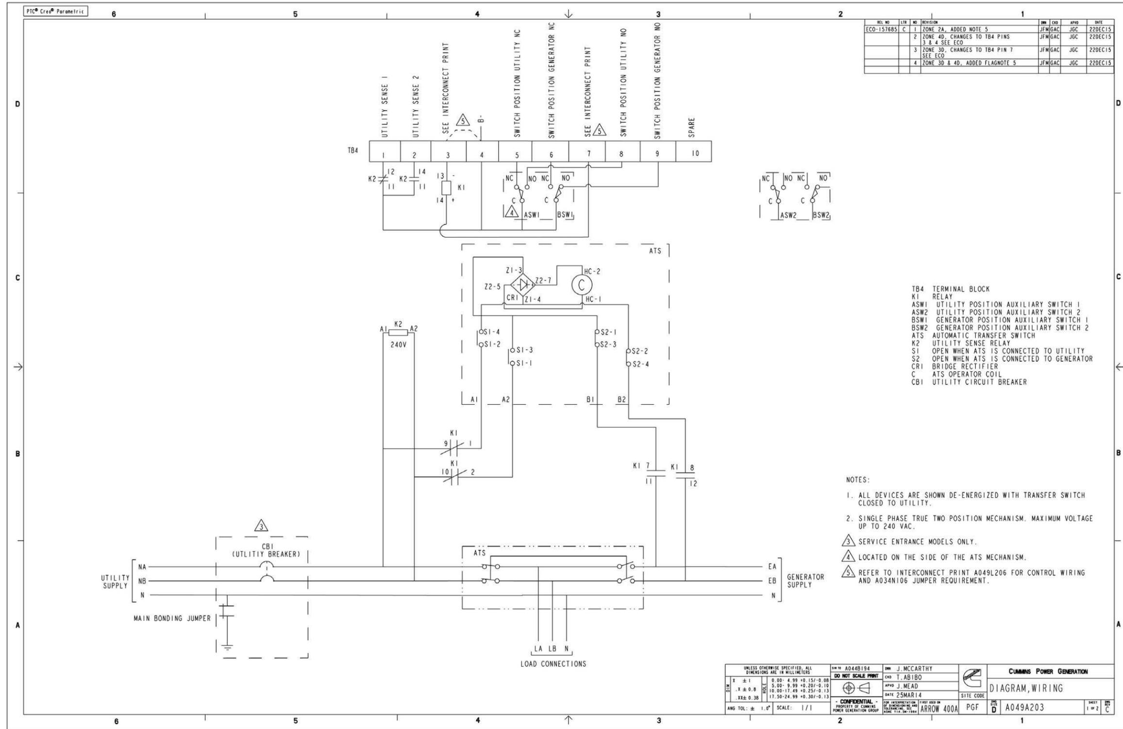
FIGURE 42. RA412N3 AND RA412S3 TRANSFER SWITCH WIRING DIAGRAM (SHEET 1 OF 2)
