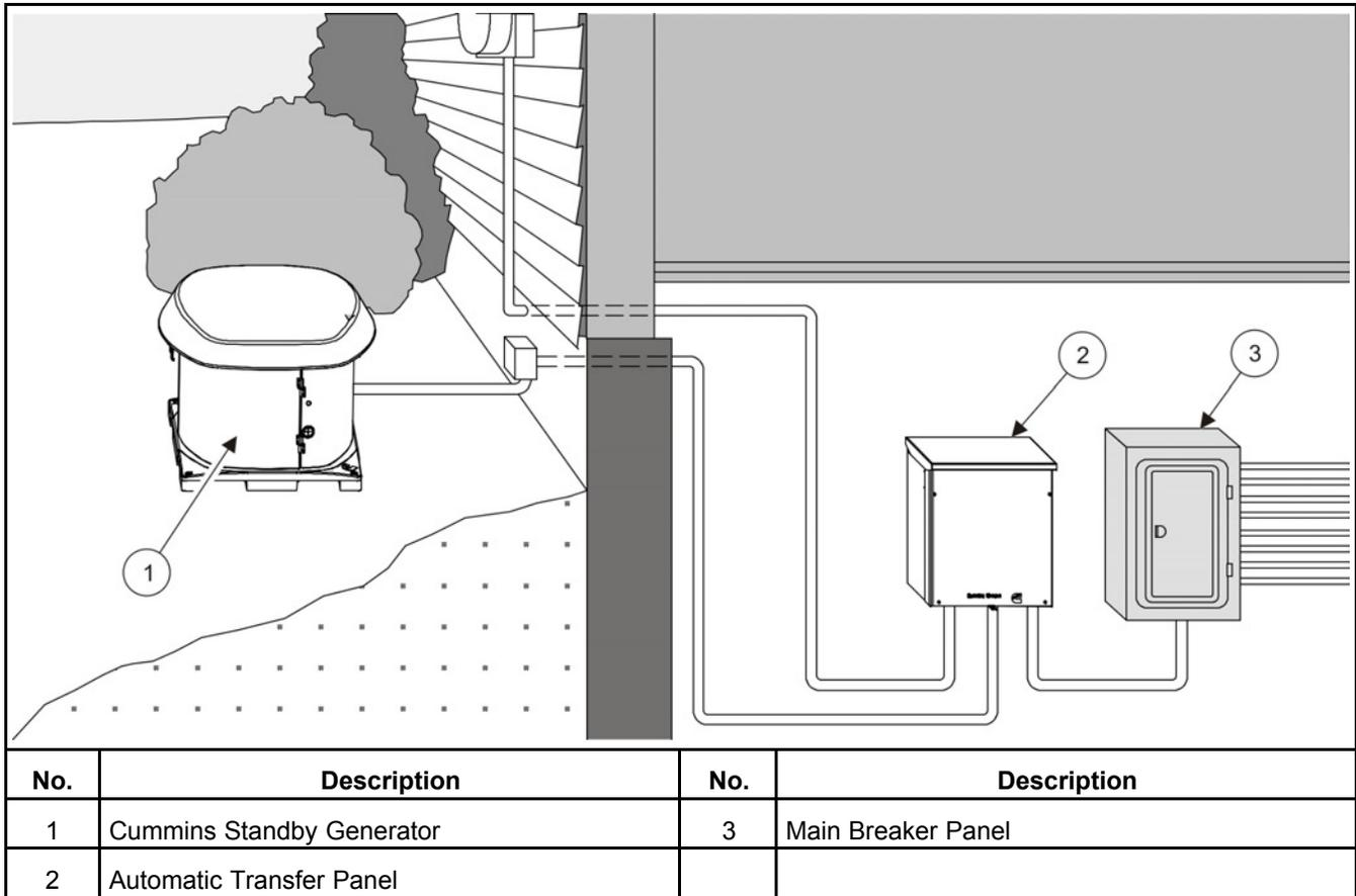
**FIGURE 19. TYPICAL WALL-MOUNT INSTALLATION OF SERVICE ENTRANCE MODELS**
