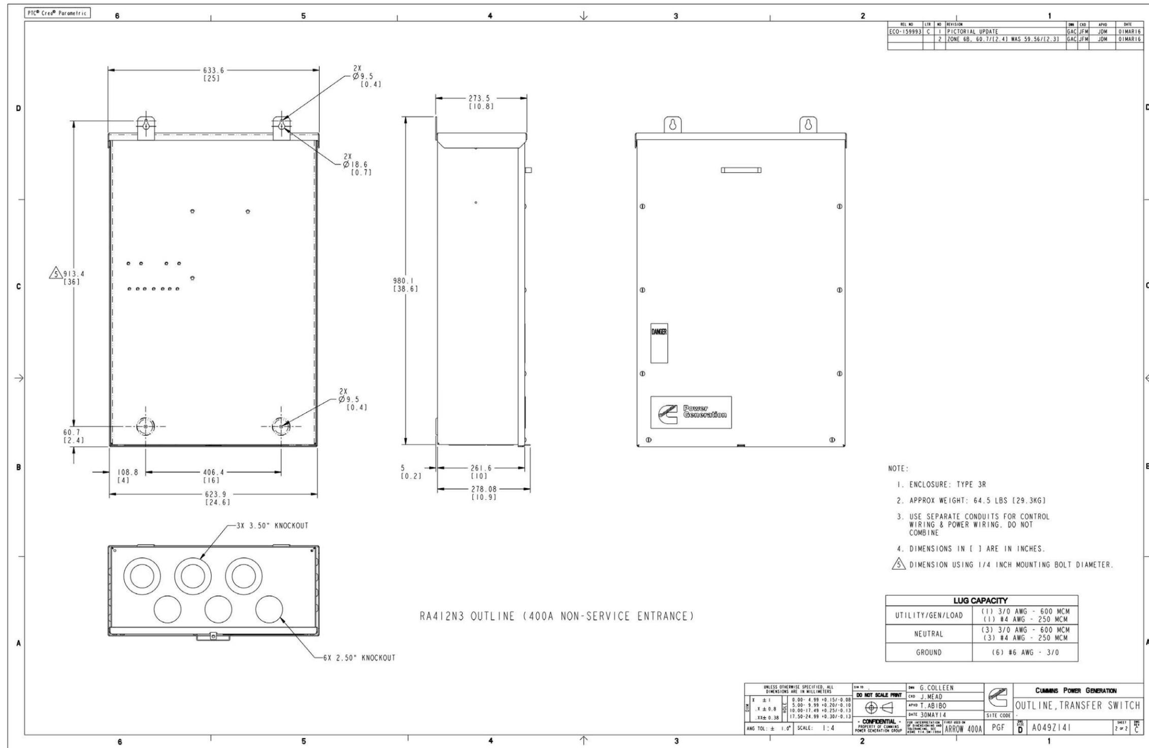
FIGURE 52. RA412N3 CONTROL BOX OUTLINE DRAWING
