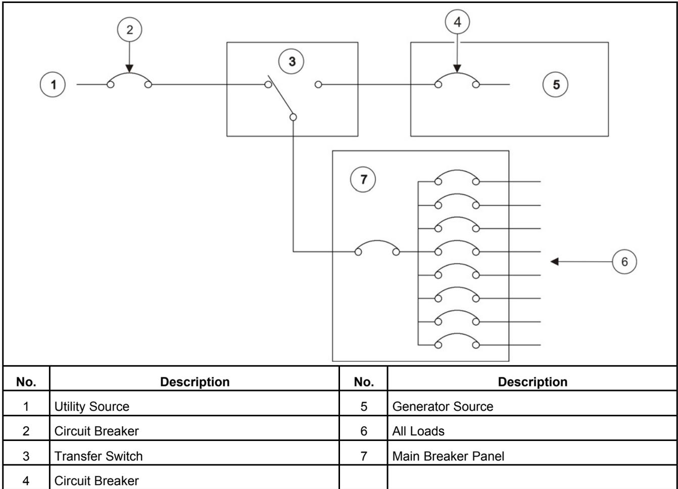
**FIGURE 16. TOTAL COVERAGE SYSTEM (NON-SERVICE ENTRANCE MODEL)**
