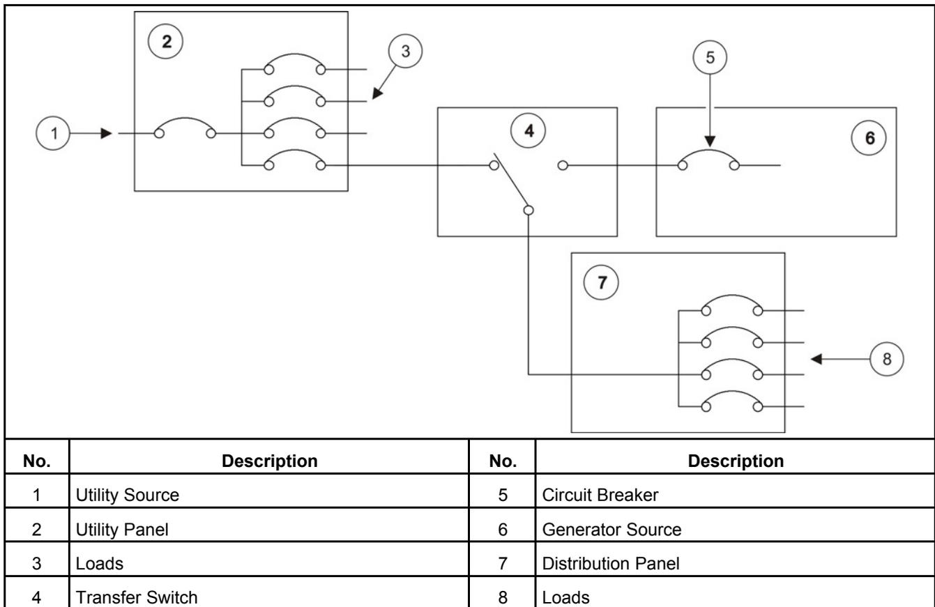
**FIGURE 14. PARTIAL COVERAGE SYSTEM (NON-SERVICE ENTRANCE MODEL)**
