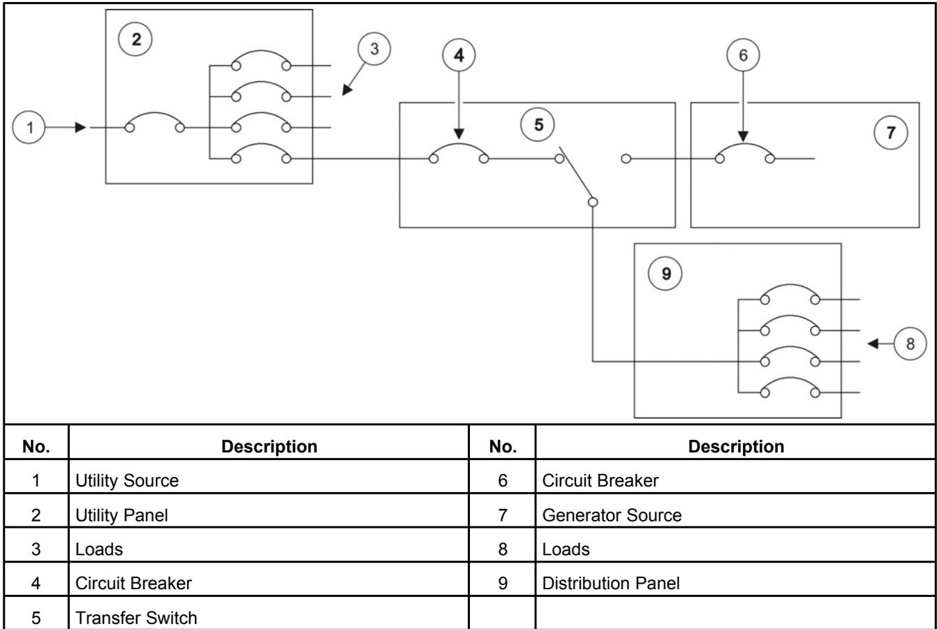
**FIGURE 15. PARTIAL COVERAGE SYSTEM (SERVICE ENTRANCE MODEL)**
