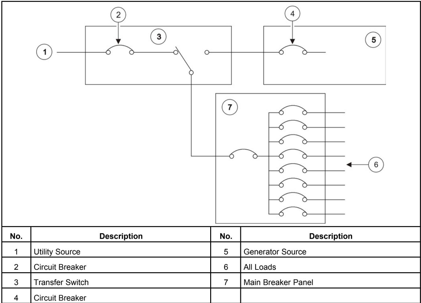
**FIGURE 18. TOTAL COVERAGE SYSTEM (SERVICE ENTRANCE MODEL)**
