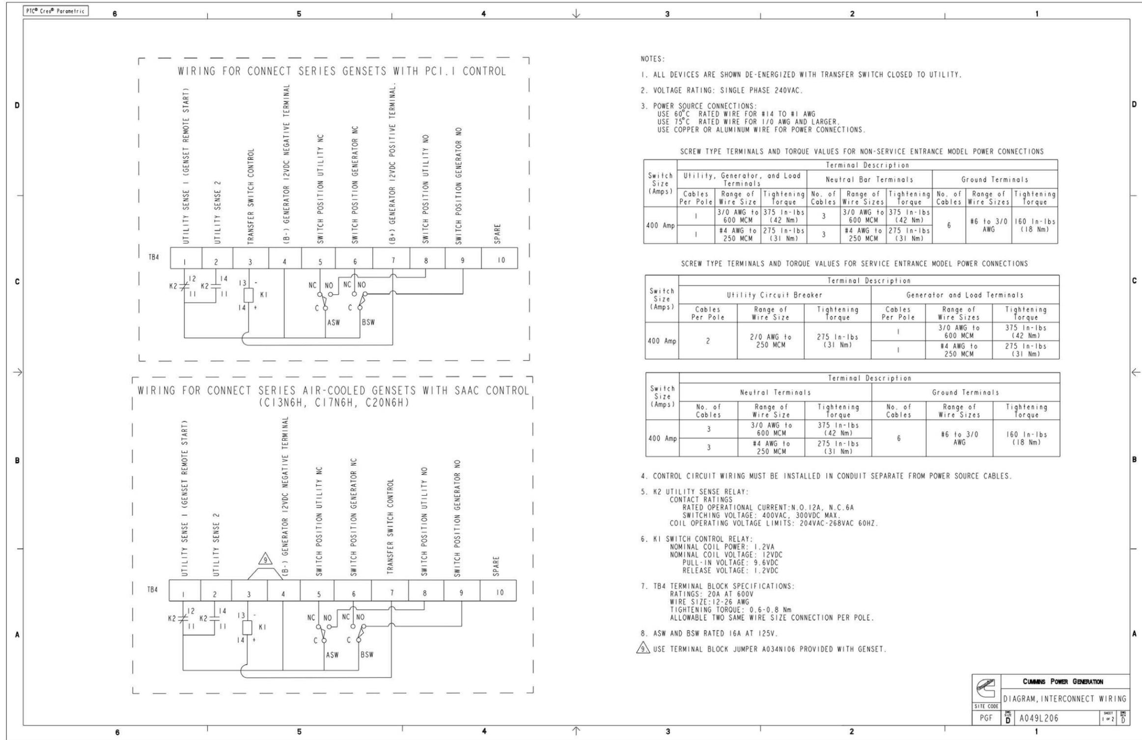
FIGURE 47. RA412N3 AND RA412S3 TRANSFER SWITCH INTERCONNECTIONS (SHEET 1 OF 2)
