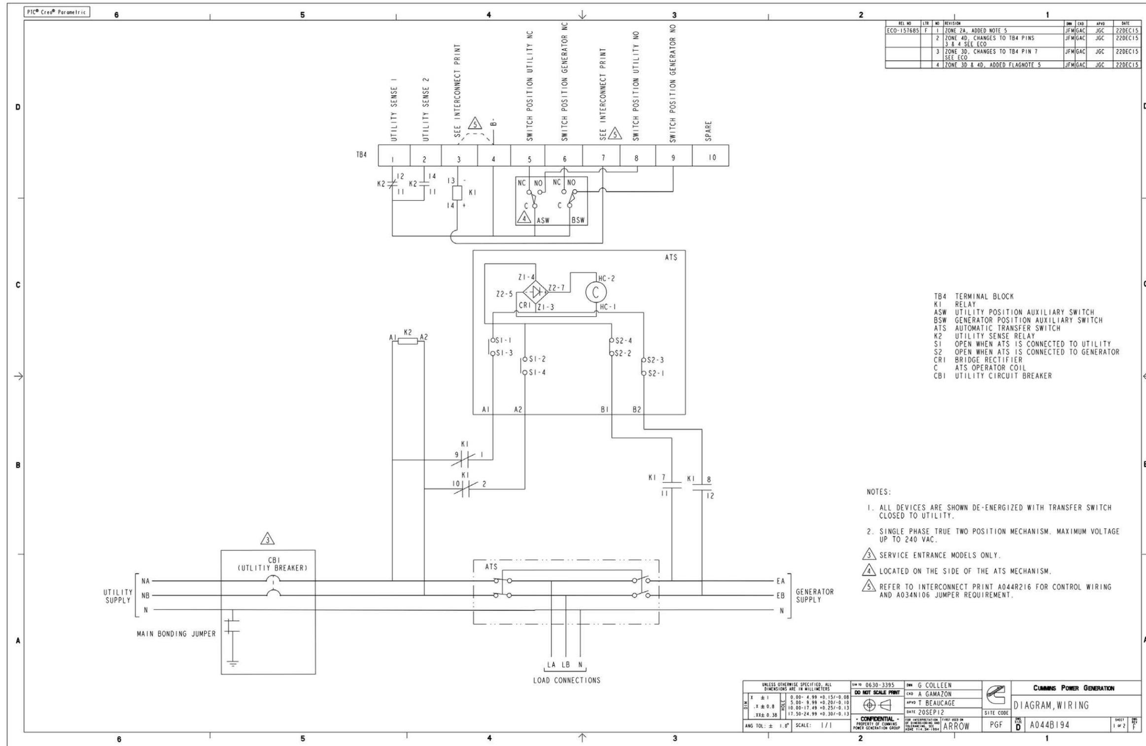
FIGURE 40. RA112N3, RA212N3, RA112S3, AND RA212S3 TRANSFER SWITCH WIRING DIAGRAM (SHEET 1 OF 2)
