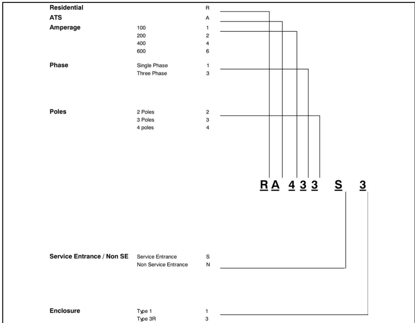
**FIGURE 6. RA SERIES TRANSFER SWITCH MODEL CHARACTER KEY**
