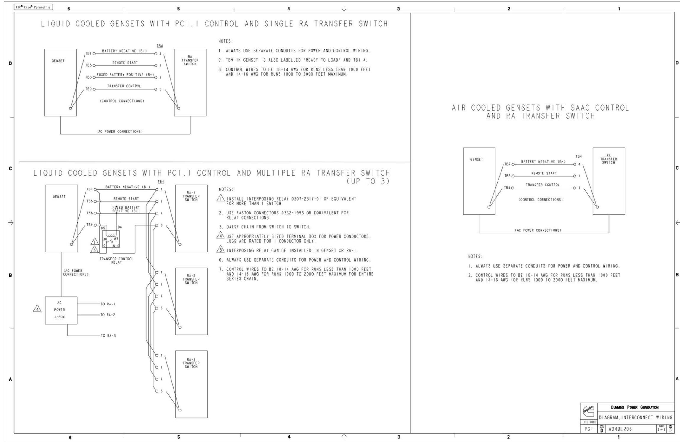
FIGURE 48. RA412N3 AND RA412S3 TRANSFER SWITCH INTERCONNECTIONS (SHEET 2 OF 2)
