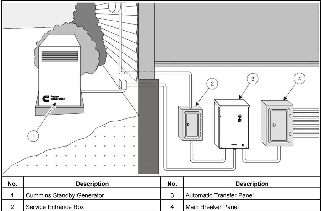
**FIGURE 17. TYPICAL WALL-MOUNT INSTALLATION OF NON-SERVICE ENTRANCE MODELS**
