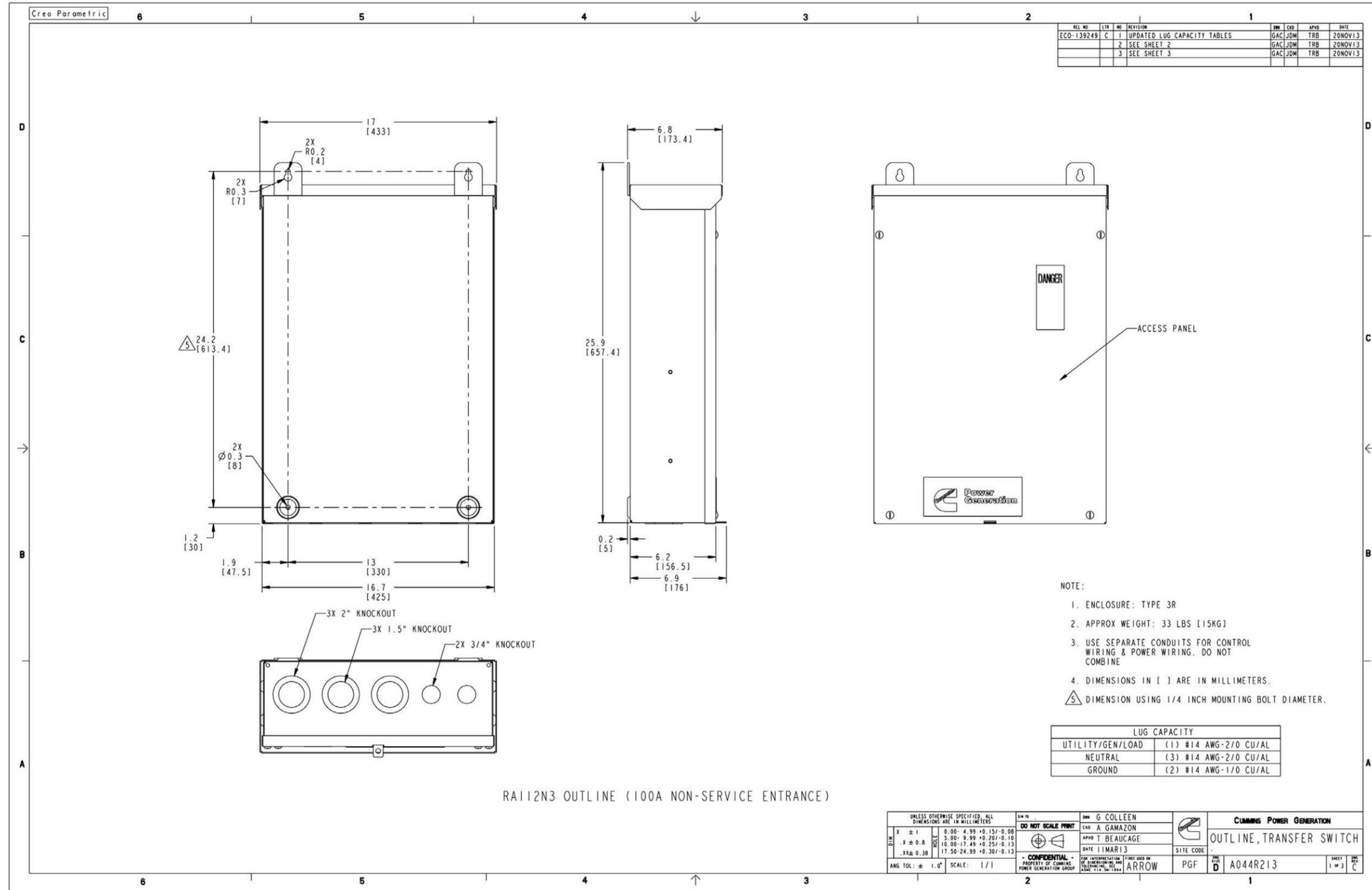
FIGURE 49. RA112N3 CONTROL BOX OUTLINE DRAWING
