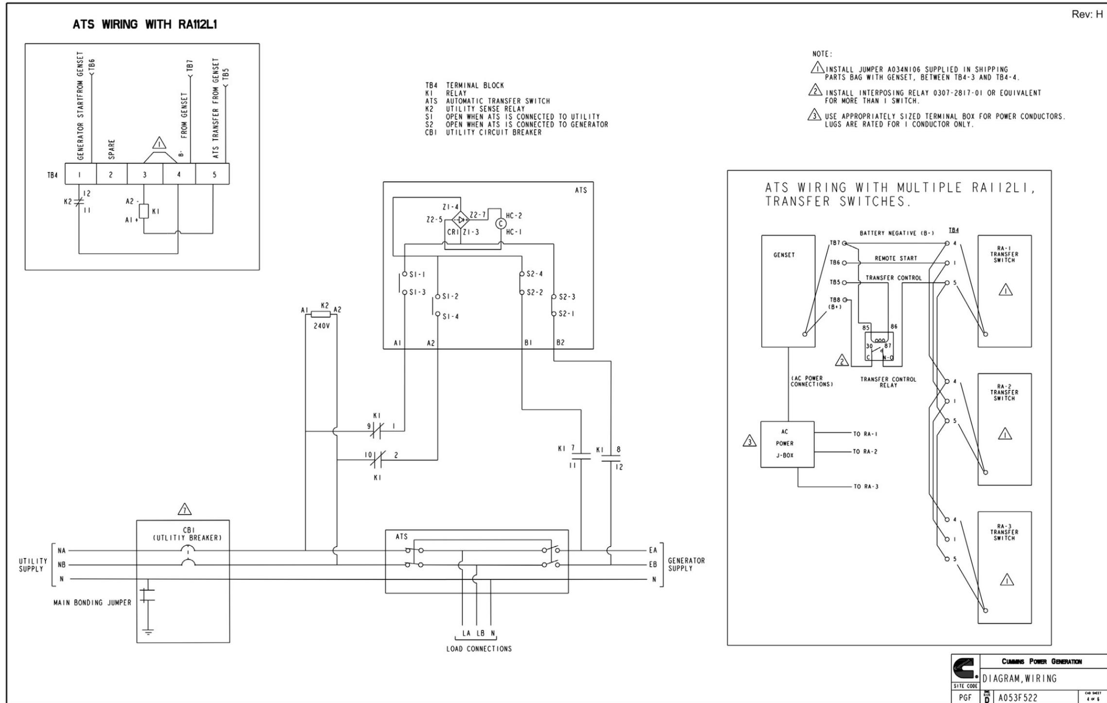
FIGURE 45. WIRING DIAGRAM (SHEET 4 OF 6)
