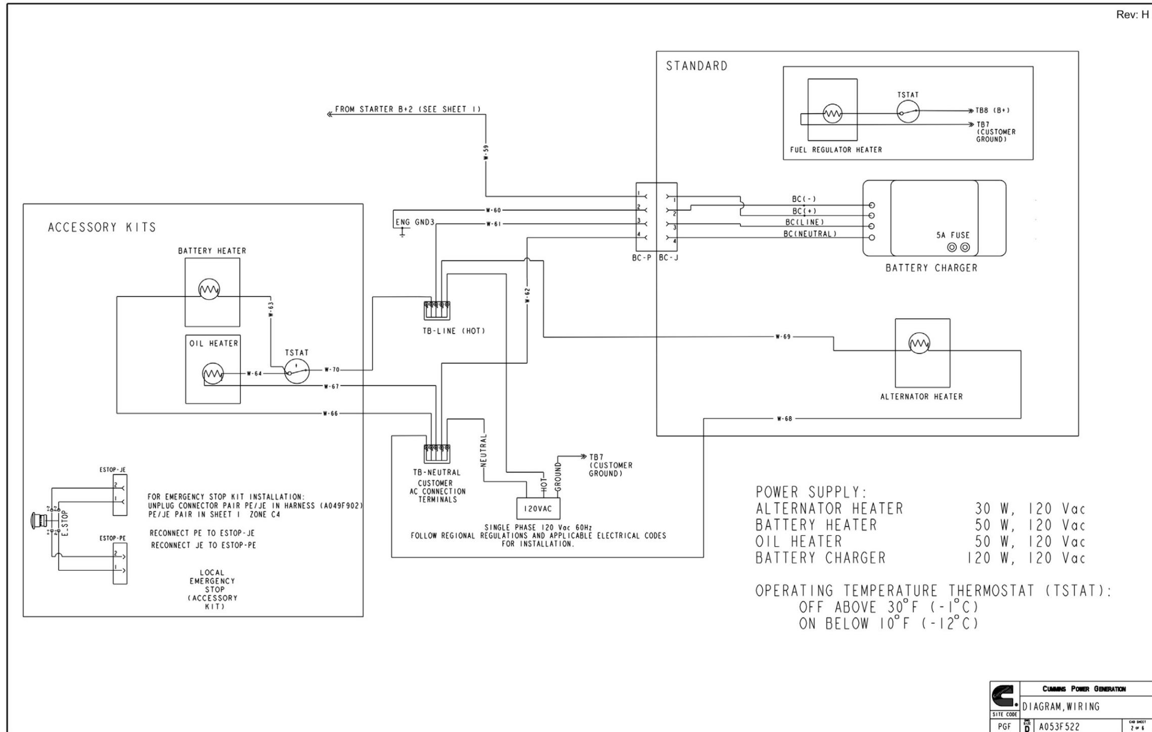
FIGURE 43. WIRING DIAGRAM (SHEET 2 OF 6)
