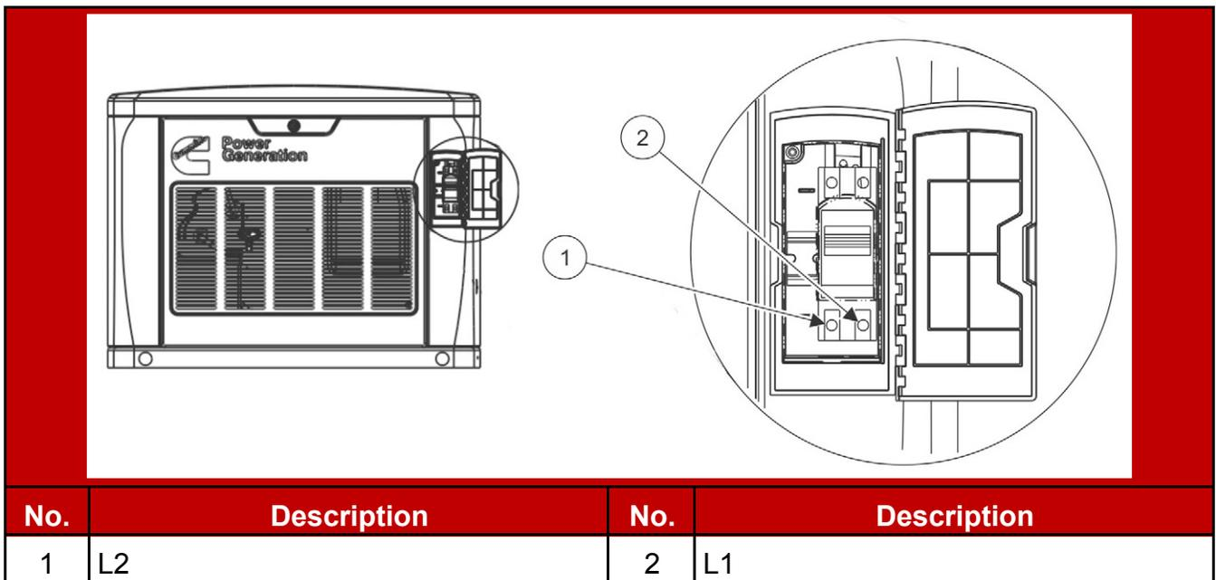
**FIGURE 13. CIRCUIT BREAKER AC LOAD CONNECTIONS LOCATION**
