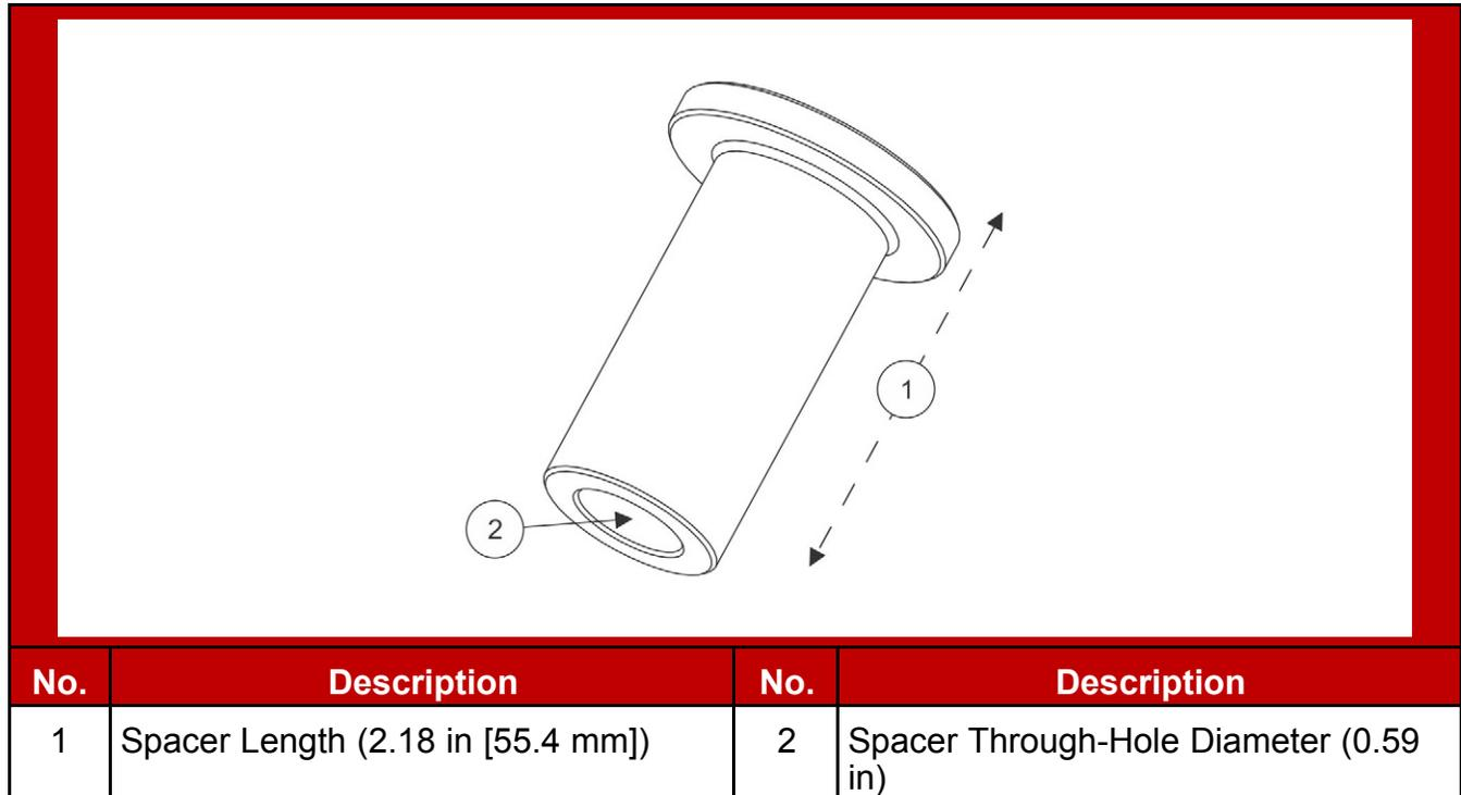
**FIGURE 5. MOUNTING SPACER**
